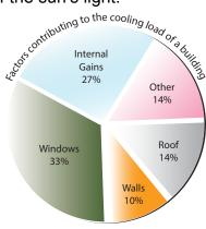
It is safe to conclude that even if the white coatings reflected 100% of the visible light, **which they do not**, the majority of the heat causing energy is getting into the structures unabated. Since the combination of the visibile light and infrared rays equals 96% of the heat energy source, restricting a major portion of these factors make it possible to acheive 50% or more in energy savings.
